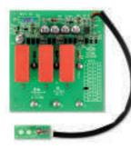
An electronic device controls (*Intelligence Device*) the status of the interlocked socket, monitoring the electrical functionality:
